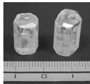
Figure 3 Large crystals of sodium ammonium tartrate prepared by the seeding method. Left, (–)-enantiomer; right, (+)-enantiomer: the pictures are taken for the crystals prepared about 25 years ago and stored as described in the text.
